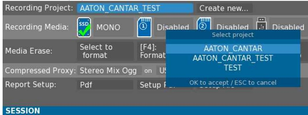
Select the current recording Project through the List build from the first enabled recording media.
