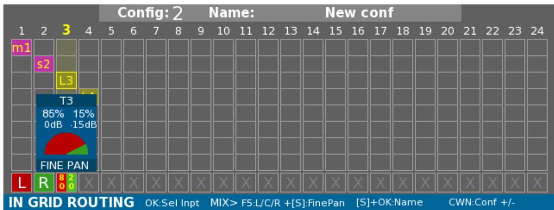
Balance is set using Left and Right keys, each track contribution will be displayed in percentage and dB.
