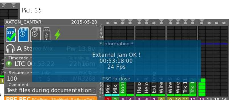
Jam has no effect if there is no valid timecode on the TC input, 'Jam Failed' appears.
