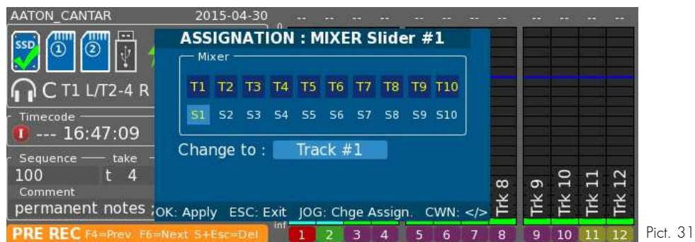
Assignment is changed by pressing Up and Down keys.
